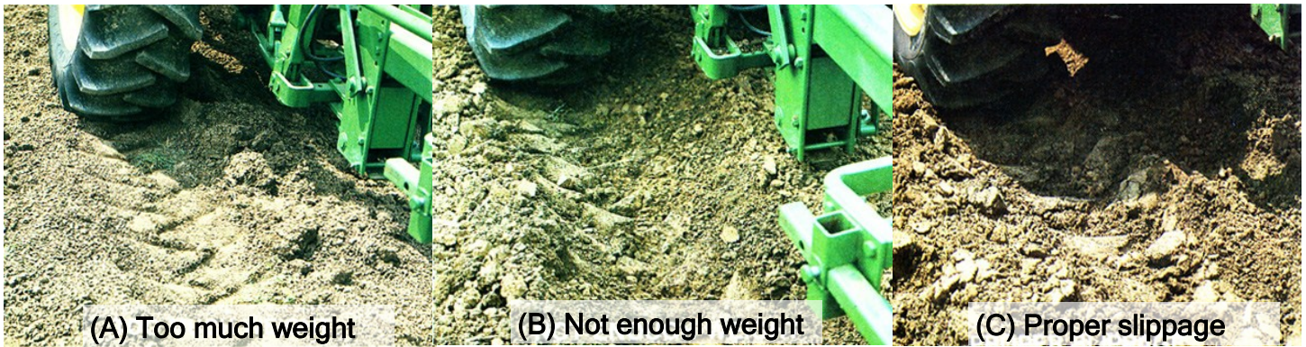
Figure 8. The footprint of a loaded tractor showing different amounts of wheel slippage. Reading footprints in the soil can tell us a lot about the object that made them. The wheels of other rolling implements like planters also have slippage, which must be factored into their calibration. Source: adapted from John Deere Service Publ., 1976.
