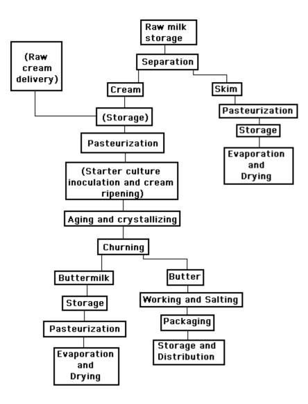
The buttermaking process involves quite a number of stages. The <u>continuous</u> <u>buttermaker</u> has become the most common type of equipment used.
