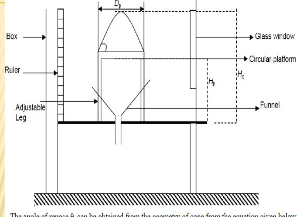
The angle of repose  $\theta_r$  can be obtained from the geometry of cone from the equation given below:  $\theta r = \tan^{-1} \left[ 2 \frac{(Hc - Hp)}{Dp} \right]$
